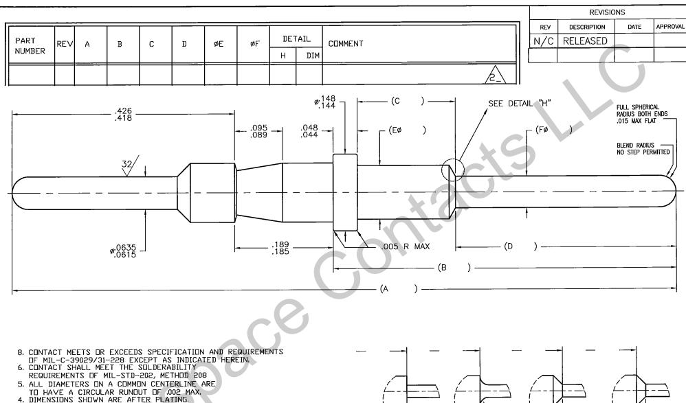
3. FINISH: .000050 THICK MINIMUM GDLD PER MIL-G45204, TYPE II, GRADE C, CLASS 1 DVER .000050-.000100 THICK SULFAMATE NICKEL PER QQ-N-290, CLASS 2, OVER .000015 THICK MINIMUM COPPER PER MIL-C-14550.
