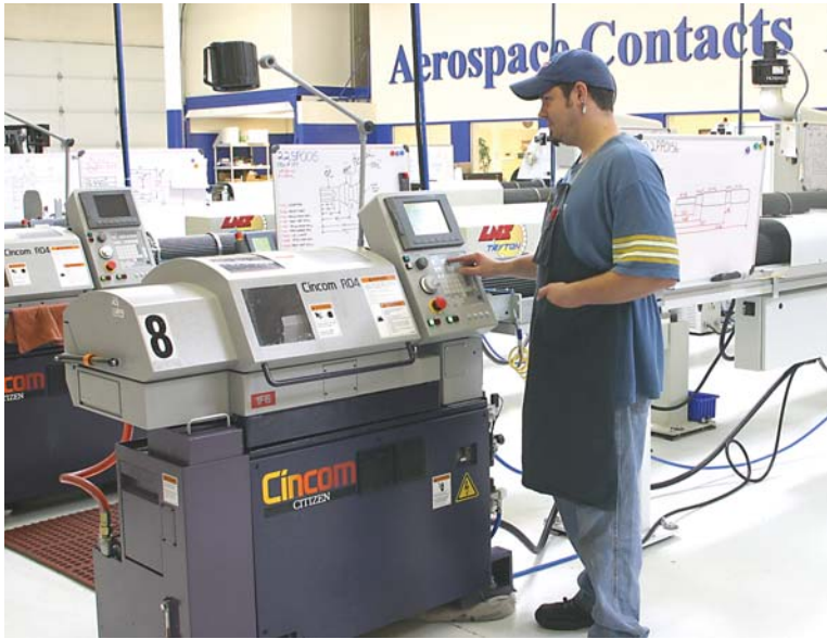
Screw machine operator Jessie Bright sets up one of Aerospace Contacts' 7 Cincom R04 series machines. The machines operate 24/7, with 4 hours of lights-out running daily.
