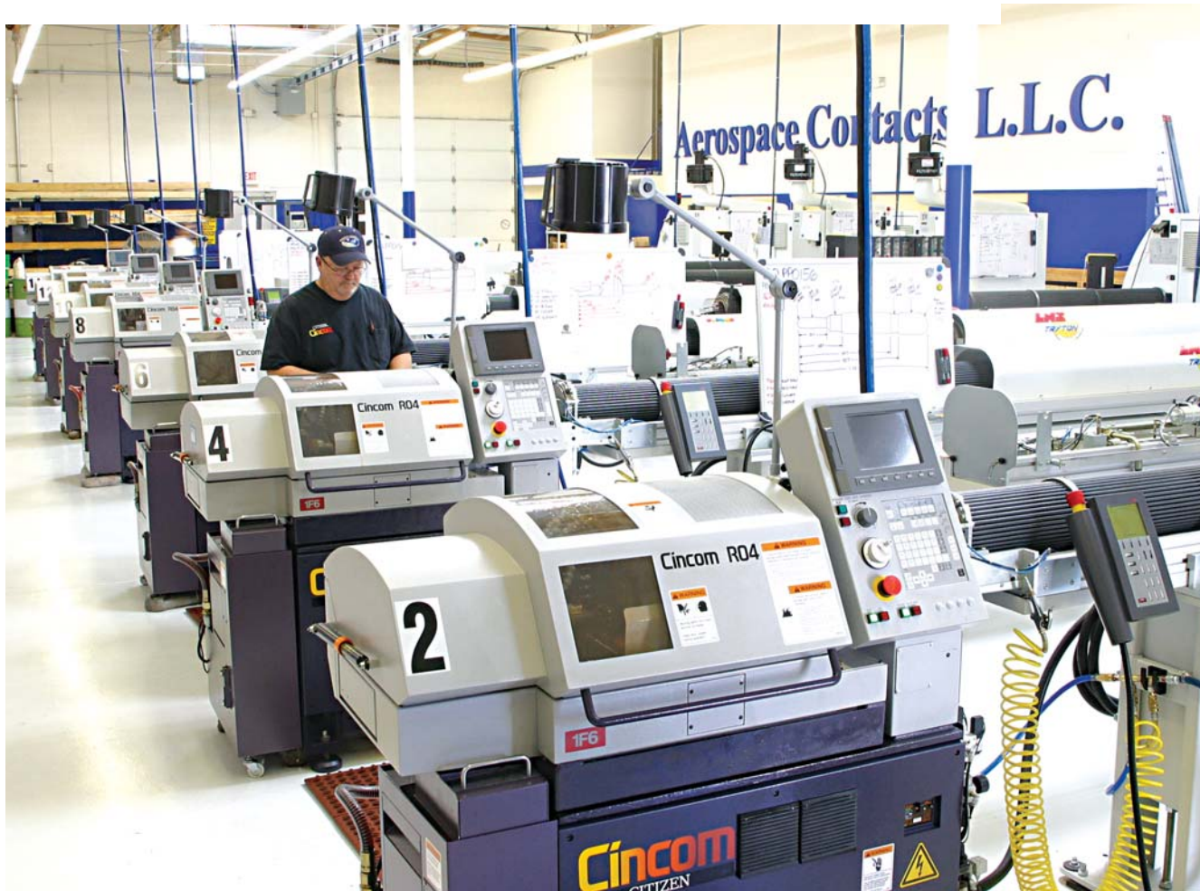
Aerospace Contacts operates 7 Citizen Cincom R04 VI model screw machines, equipped with LNS Tryton automated bar feeders. The machines run 24/7 including 4 hours a day lights out. The company runs two full-time and one half-time shift. Operator in photo is Dick Waters, machine shop supervisor.
